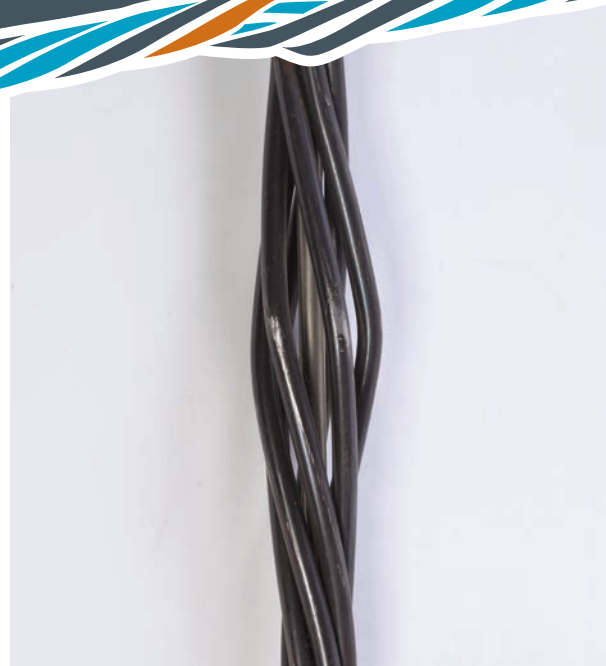
SMART cables are indistinguishable from regular cable bolts in the bond section.
