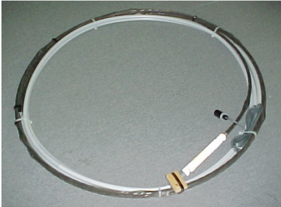
Photo 1: Coiled SMART cable as it arrives on site.
